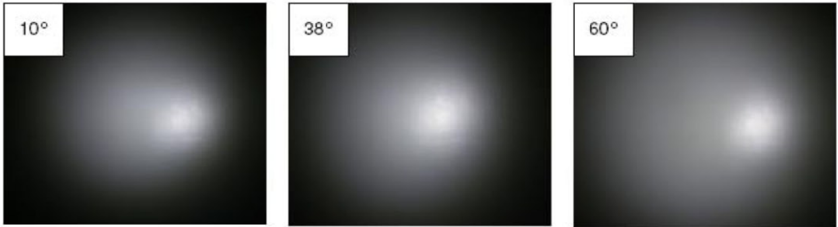
< Figure 11 Different beam angle from 1 meter picture >
