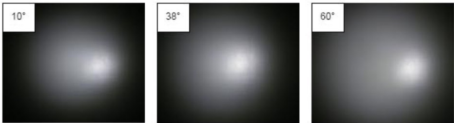
< Figure 11 Different beam angle from 1 meter picture >
