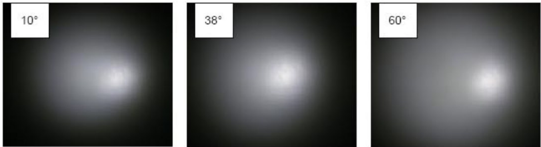
< Figure 11 Different beam angle from 1 meter picture >
